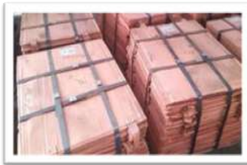
Figure 8: Typical copper cathodes
